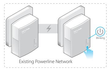
2 Press the Pair button on the new adapter.
