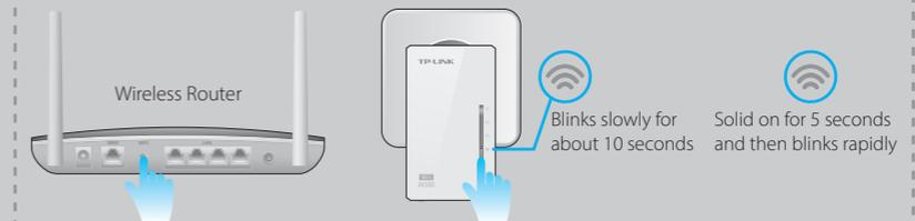
**Note:** If the Wi-Fi LED still blinks slowly for longer than 30 seconds, unplug the extender and plug it back in, then try again. Or use "Customize the Extender's Wi-Fi Settings" on the back instead.
