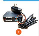
Connect the charger to the Cisco power port and to the electrical outlet
