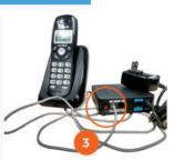
Connect the Rj11 cable from the phone to port 1 of the Cisco
