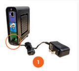
Connect the charger to the power port of the modem and to the electrical outlet
